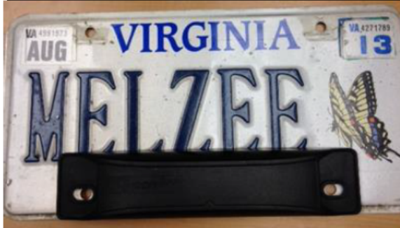
Fig- 2 Proper Mounting of Bumper E-Z Pass
